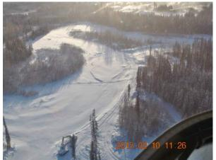
Frazil ice is believed to be a major contributor to ice accumulation in the channel, causing ice jamming on the lower reach of the Mayo River. This is accomplish by implementing flow cut back during freeze up. Furthermore, daily and hourly flow rate fluctuations are minimize to reduce frazil ice transport and to minimize the potential of collapsing or breakage of the ice cover as a result of flow changes.
